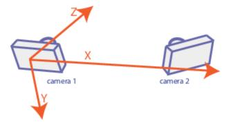
When you reconstruct a 3-D scene using a calibrated stereo camera, the reconstructScene and triangulate functions return 3-D points with the origin at the optical center of Camera 1. When you use Kinect<sup>®</sup> images, the pcfromkinect function returns 3-D points with the origin at the center of the RGB camera.
