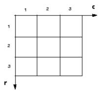
For pixel coordinates, the number of rows, r, downward, while the number of columns, c, increase to the right. Pixel coordinates are integer values and range from 1 to the length of the row or column. The pixel coordinates used in Computer Vision Toolbox software are one-based, consistent with the pixel coordinates used by Image Processing Toolbox<sup>™</sup> and MATLAB. For more information on the pixel coordinate system, see "Pixel Indices".
